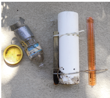
One of the University of Florida-manufactured crazy ant traps. The bottle contains food, water and traces of pesticide. Holes along the bottom of the PVC offer ants access.
